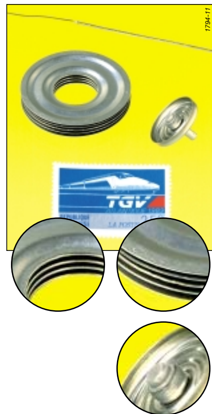
Welding membranes and thermocouple junctions.
